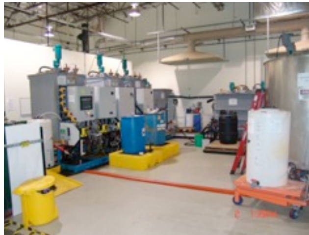
5 gpm pilot system with adjustable retention times
